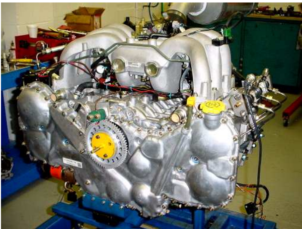
Figure 6 6-Cylinder Subaru SCS SCAI HFE with Direct Injection, Common Rail
