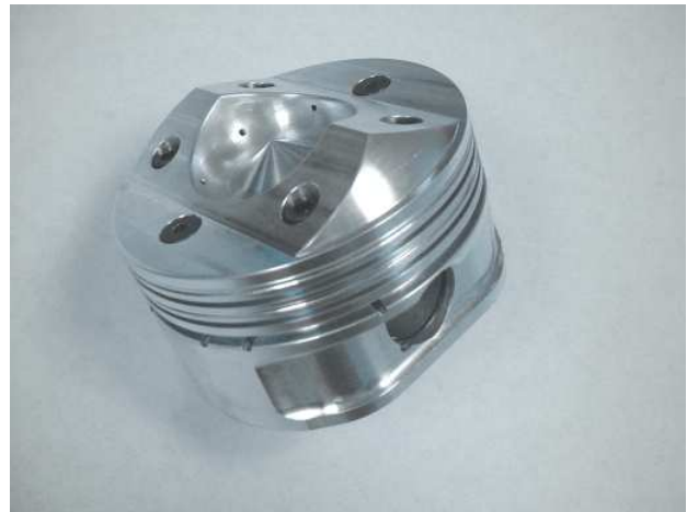
Figure 7 Subaru SCS SCAI HFE Preliminary Piston
