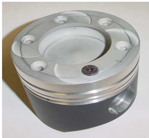
Figure 8 250 Hp SCAI HFE Improved Piston
