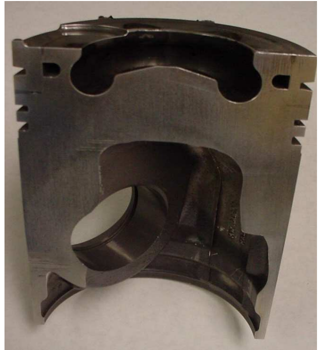
Figure 3 SCS ELECTRON BEAM WELDED PRE-PRODUCTION PISTON
